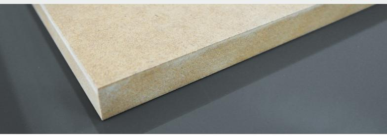
MDF, also called medium-density fiberboard, is made of pressed conifer wood fibers, and is used in the furniture sector for carcasses, drawers and fronts. Moreover, MDF is also used as base material for desks or cabinet systems. Because of the high bending- and tensile-strength and the smooth surface, the fiberboard is very popular.
